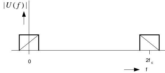
Figure 3.6: Spectrum of u(t) (see equation 3.13). A channel transfer function H(f) = 1 \forall f is used for simplicity
